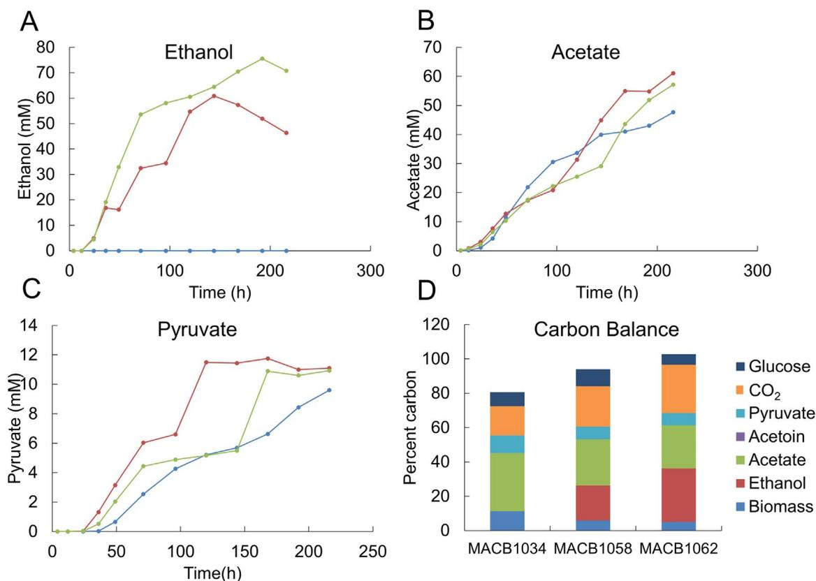
**Fig. 6.** Acetate (A), ethanol (B), and pyruvate (C) production and carbon balances (D) for cultures grown in 1 L bioreactors with crystalline cellulose as the carbon source at 60 °C for strains MACB1034 (blue), MACB1058 (red), and MACB1062 (green). Carbon balances were calculated based on measured glucose, pyruvate, acetoin, acetate, ethanol, cellular protein (biomass) and residual Avicel.
