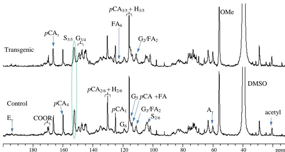
**FIGURE 2 | Quantitative  $^{13}\text{C}$  NMR spectra of enzyme lignins isolated from switchgrass internode I1 samples (Bottom: control; top: transgenic).** A,  $\beta$ -O-4; G, guaiacyl; S, syringyl; H, *p*-hydroxyphenyl; *p*CA, *p*-coumarate; FA, ferulate; E, cinnamyl aldehyde; OMe, methoxyl.
