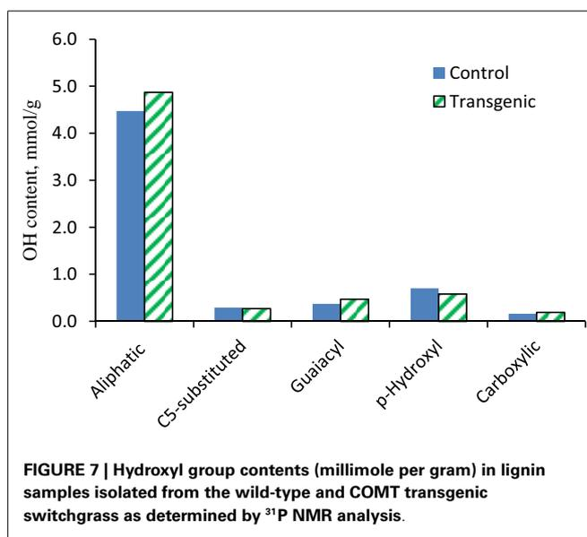
**FIGURE 7 | Hydroxyl group contents (millimole per gram) in lignin samples isolated from the wild-type and COMT transgenic switchgrass as determined by  $^{31}\text{P}$  NMR analysis.**
