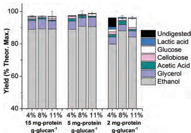
Fig. 4 Theoretical yields of ethanol, glucose, and glucose derived by-products from SSF of CELF pretreated corn stover solids over the range of glucan and enzyme loadings (*i.e.*, mg-protein per g-glucan-in-RCS).
