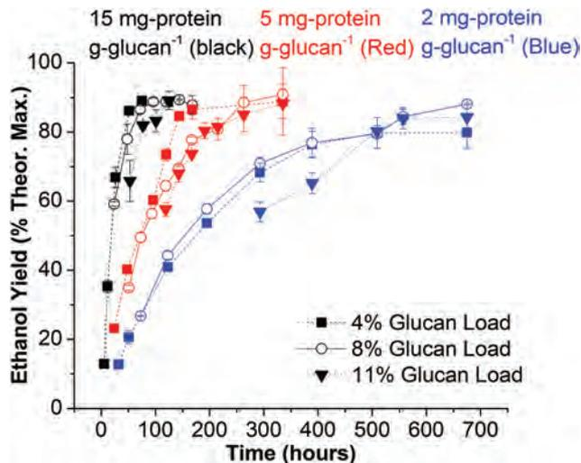
Fig. 3 The effect of enzyme loadings at 2, 5, and 15 mg-protein per g-glucan-in-RCS on SSF fermentation times and ethanol yields for CELF solids at glucan loadings of 4, 8, and 11 wt%.
