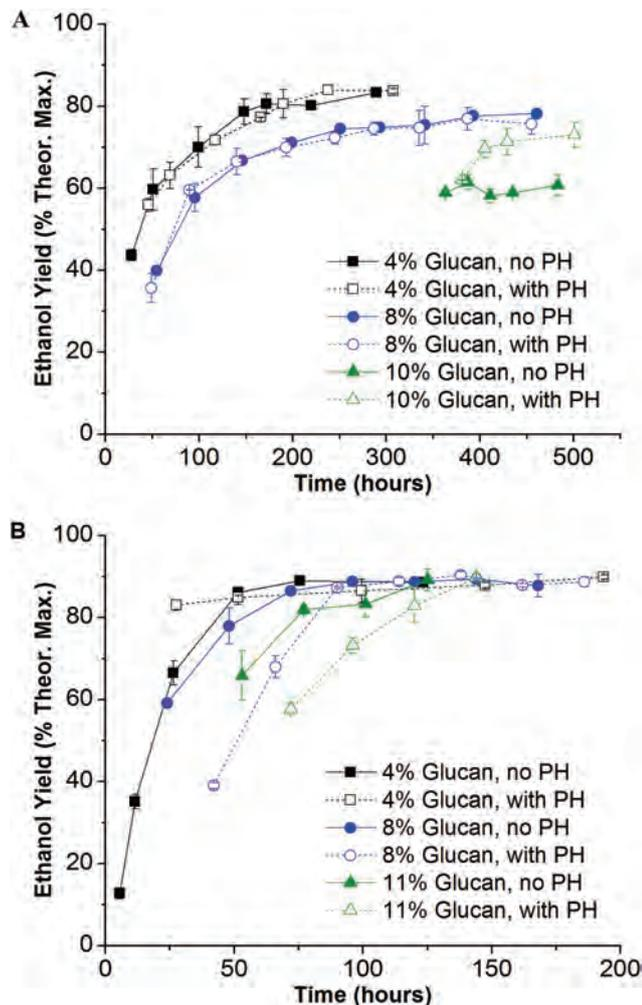
Fig. 2 Effects of glucan loading and 18 h prehydrolysis (PH) at 50 °C on percent ethanol yields of theoretical maximum for SSF of solids from (A) DA and (B) CELF pretreatments of corn stover. Accellerase® 1500 enzyme loading of 15 mg-protein per g-glucan-in-RCS. Fermentations without PH are shown as solid lines, while fermentations with PH are shown as dashed lines. The times include the time for the PH step when appropriate.
