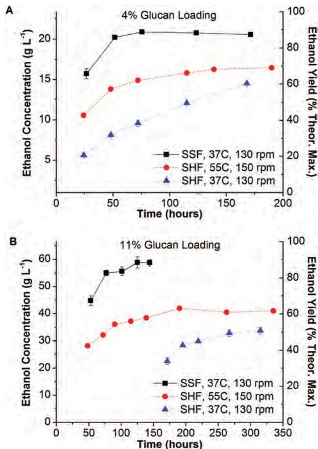
**Fig. 1** Comparison of percent ethanol yields of theoretical maximum and concentrations ( $\text{g L}^{-1}$ ) for SSF and SHF at 37 °C and 55 °C for CELF pretreated solids at (A) 4 wt% and (B) 11 wt% glucan loadings and a cellulase loading of 15 mg-protein per g-glucan-in-RCS. For SHF, ethanol yields and concentrations are calculated values based on 90% of theoretical maximum ethanol possible.
